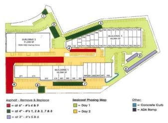
Site plans are critical to making sure you know exactly where the repair locations are and what the dimensions of the repairs will be.
